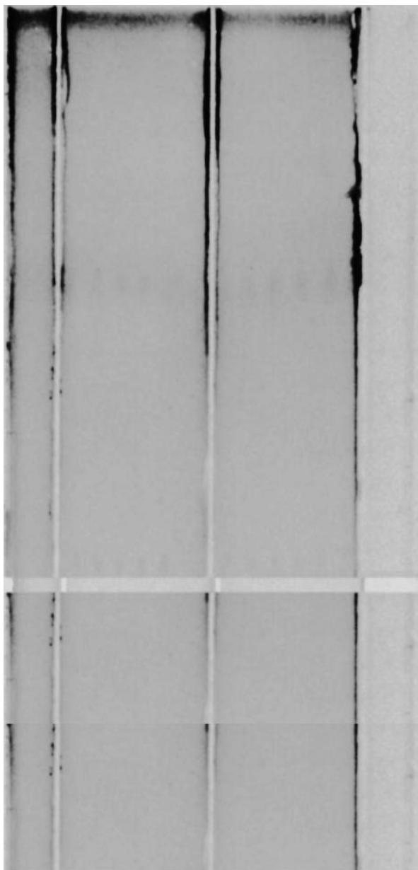
Figure 2. OPTIC separation of the neutral lipid classes. 2.a plate, 2.b densitogram of one lane, NGL = neutral glycolipids, Ch = cholesterol, Glyc = glycerides, ChE = cholesterol esters. Plate Merck HPTLC Si 60, 17 cm elution with chloroform.
